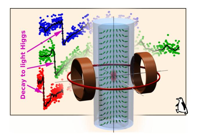
Helium-3 experimental cell and extract of data showing creation of light Higgs mode (analog of 125 GeV Higgs boson). Credit: Dr. Vladislav Zavyalov, Low Temperature Laboratory, Aalto University
