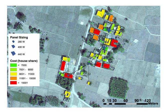
Figure 2: This GridForm model of a village in Bihar, India, shows the optimal layout of hardware for the load profiles of the community. Each building, color-coded by the cost (in Indian rupees) of supplying electricity to that structure, is wired to a central generation/storage node (solid lines), and the nodes are connected to each other (dotted lines).
