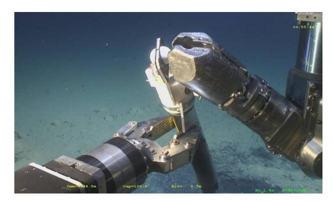
A remotely-operated vehicle collects a sediment core from deep ocean waters offshore of the Congo River mouth in 2011. Credit Georgia Institute of Technology.
