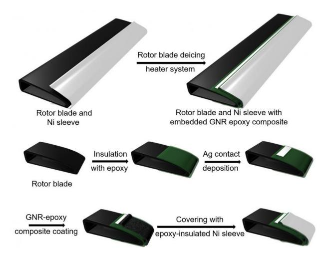
Lab tests at Rice University on a section of a helicopter rotor chilled to minus-4 degrees Fahrenheit show that a thin coat of nanoribbon-infused epoxy can be used as a de-icer. The composite, imbedded between an abrasion shield and the blade in the sample above, heated when electricity was applied, melting the ice. The material may be suitable for keeping aircraft, wind turbines and transmission lines free of ice. Credit: Tour Group/Rice University
