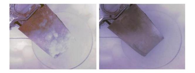
Rice University scientists embedded graphene nanoribbon-infused epoxy in a section of helicopter blade to test its ability to remove ice through Joule heating. Credit: Tour Group/Rice University
