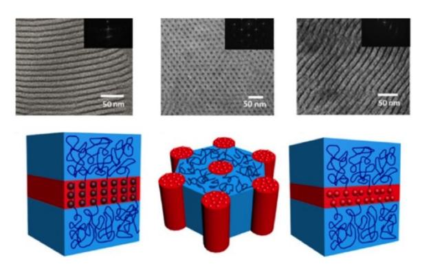
Depending on the relative amounts of different building-block molecules, it is possible to create different sandwich and wheel topologies (shown above in micrographs and below as models). Credit: American Chemical Society. Copyright 2016
