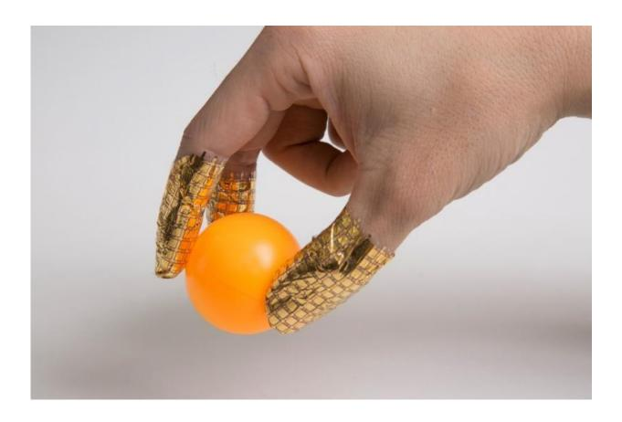
The pressure sensors wrap around and conform to the shape of the fingers while still accurately measuring pressure distribution. Credit: 2016 Someya Laboratory
