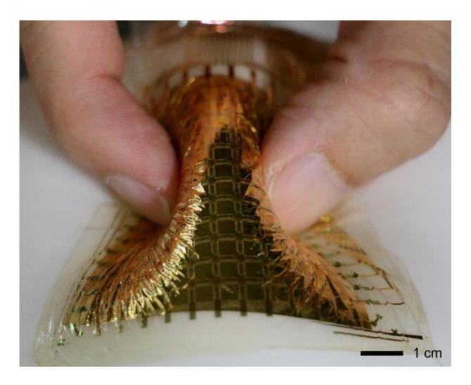
The flexible pressure sensor conforms to the shape of an inflated balloon. Even when the sensor is stretched and deformed with the shape of the balloon, the device still measures the pressure distribution accurately. Credit: 2016 Someya Laboratory
