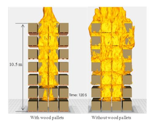
Stacking commodities on wood pallets (left image) slows horizontal fire spread, versus absence of pallets (right image).
