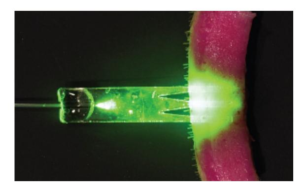
Bioabsorbable optical waveguides can be implanted into tissue to deliver light deeper and more effectively. After use, there is no need for removal as the waveguide disappears over time.
