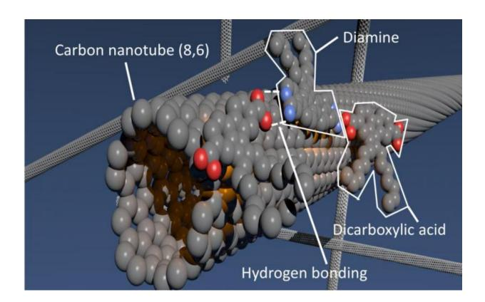
Hydrogen bonding allows a fluorene based polymer to grow on specific carbon nanotubes. This changes the solubility of the nanotube allowing it to be separated from other types of nanotubes. Credit: International Institute for Carbon-Neutral Energy Research (I<sup>2</sup>CNER), Kyushu University
