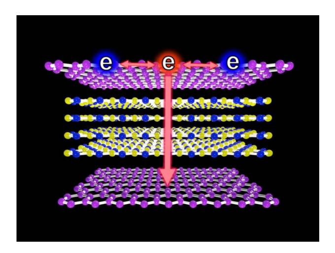
An illustration showing single layers of graphene with thin layers of insulating boron nitride that form a sandwich structure. Credit: Qiong Ma
