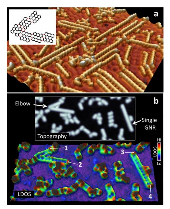
Figure 1 shows interconnected graphene nanoribbons (GNRs). The interconnection points are observed as elbow structures. The inset of (a) shows
