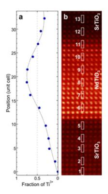
Scanning transmission electron micrograph (right) and  $Ti^3$ + fraction  $[Ti^3+/(Ti^3++Ti^4+)]$  extracted from electron energy loss spectra (left) for a  $SrTiO_3/NdTiO_3/SrTiO_3$  heterojunction. Electron transfer from  $NdTiO_3$  to  $SrTiO_3$  results in  $Ti^4$ + in the former and  $Ti^3$ + in the latter. The electrons transferred to the  $SrTiO_3$  are itinerant and constitute the highest density quasi-2D electron gas (3 × 1015 e-/cm²) ever achieved in a semiconductor superlattice.
