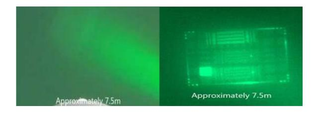
Left: an image of a chessboard pattern taken by a standard camera at a distance of 7.5 metres. Right: an image of the same object taken by the new camera prototype. Credit: SINTEF
