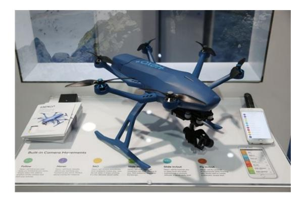
The Hexo+ Your Self-Flying Camera drone is on display at the Hexo+ booth during CES International, Thursday, Jan. 7, 2016, in Las Vegas. The fully autonomous drone has no controller. Using a smart phone app, the user selects how and from what angle you want the drone to take video of you and it will automatically follow you around with it's camera. (AP Photo/John Locher)
