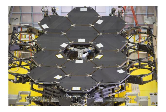
One dozen (out of 18) flight mirror segments that make up the primary mirror on NASA's James Webb Space Telescope have been installed at NASA's Goddard Space Flight Center. Credit: NASA/Chris Gunn
