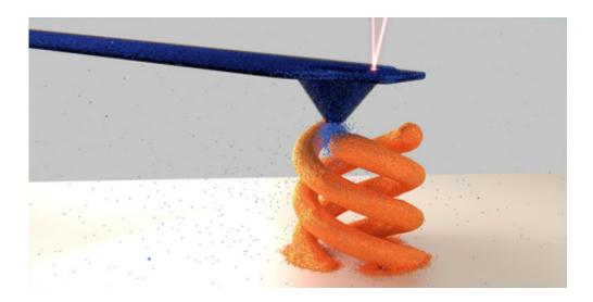
ETH researchers use a movable micropipette (blue) to manufacture tiny copper objects. Credit: ETH Zurich / Alain Reiser
