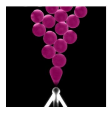
SMall 20 micron liposomes (purple bubbles) are formed by fluid flows from the nozzle. Credit: Delft University of Technology
