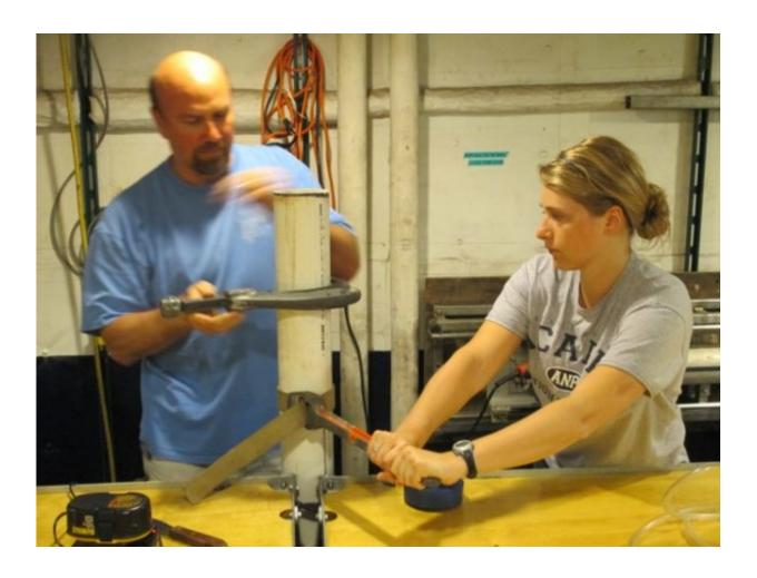
Aboard the research vessel, Steve Hovan of the Indiana University of Pennsylvania and Allison Jacobel of Lamont-Doherty Earth Observatory cut a sediment core into sections. Credit: Pratigya Polissar/Lamont-Doherty Earth Observatory
