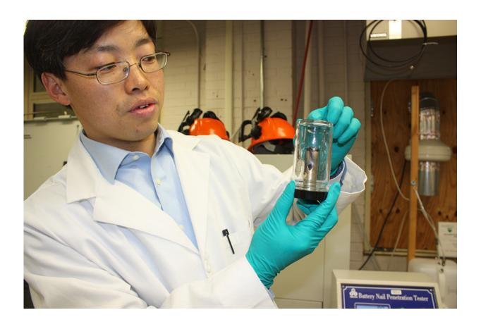
Guangsheng Zhang shows a punctured lithium-ion (Li-ion) battery. Researchers at Penn State are working to make these batteries safer. Credit: Penn State
