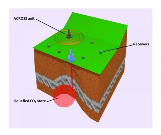
Analyzing seismic waves generated by an Accurately Controlled Routinely Operated Signal System (ACROSS) unit can reveal information about the amount and location of CO2 leakage from an underground store. Credit: International Institute for Carbon-Neutral Energy Research (I<sup>2</sup>CNER), Kyushu University
