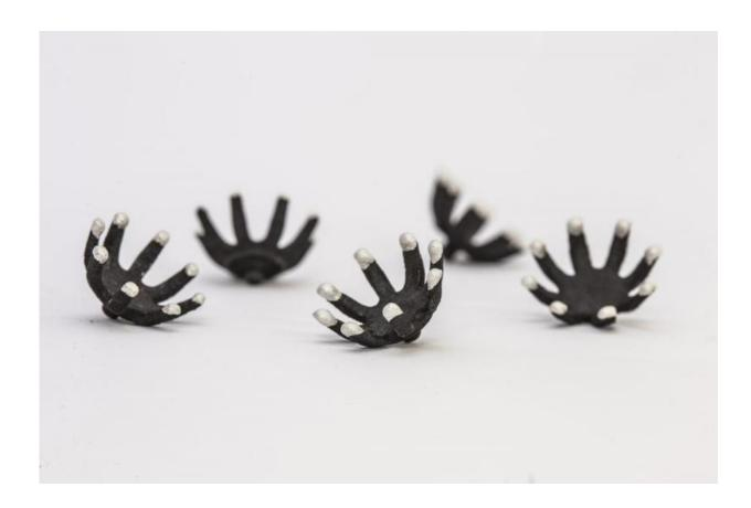
Researchers spent four years perfecting the recipe for the sensors' materials. Sensors designed to work on a subject's hair are made of a mix of silver and carbon deposited on a flexible substrate. This material allows sensors to remain flexible and durable while still conducting high-quality signals--a silver/silver-chloride coating is key here. Credit: Jacobs School of Engineering/UC San Diego
