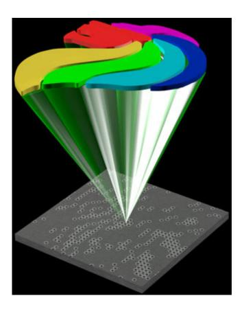
Dense arrays of light scattering nanoholes can make anti counterfeiting holograms more secure. Credit: A\*STAR Institute of Materials Research and Engineering
