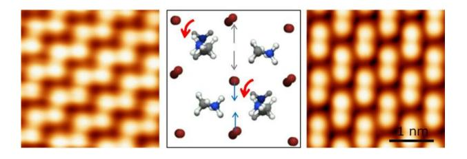
Methylammonium molecules (represented by a ball-and-stick model in the centre) in methylammonium lead bromide (CH3NH3PbBr3) can rotate. They favour specific orientations that lead to two types of surface structures with distinctly different properties (left and right images).
