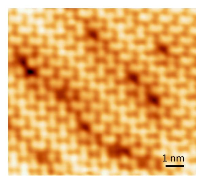
Atomic size defects on the surface of a perovskite crystal.
