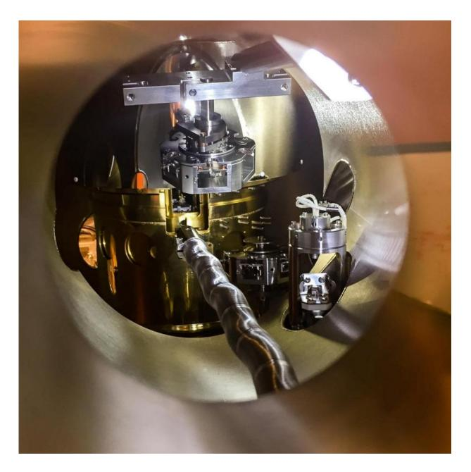
Inside view of the scanning tunneling microscope. The yellow cylinders are the heat shields, behind which the sample gets cooled.
