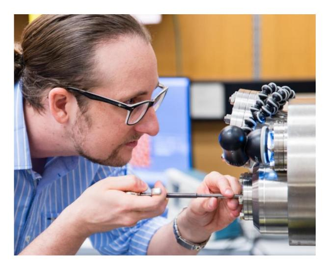
Dr Ohmann transfers a sample into the scanning tunneling microscope.
