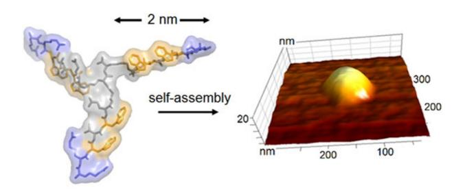
The chemical structure of the nanoscale building block (left) and its assembly into a virus-like capsule (right, topographic AFM image)
