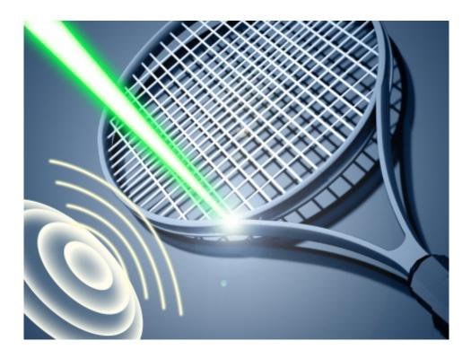
The research team have developed the first demonstration of 3D printing of composite materials. Ultrasonic waves produce a pattern of microscopic glass fibres which give the component increased strength. A laser cures the epoxy resin and creates the component. Credit: Matt Sutton, Tom Llewellyn-Jones and Bruce Drinkwater
