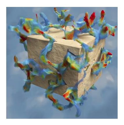
Simulated fluid flow in a small sub-volume. Red and blue arrows indicate fast and slow flow velocities while yellow and green arrows represent intermediate velocities.
