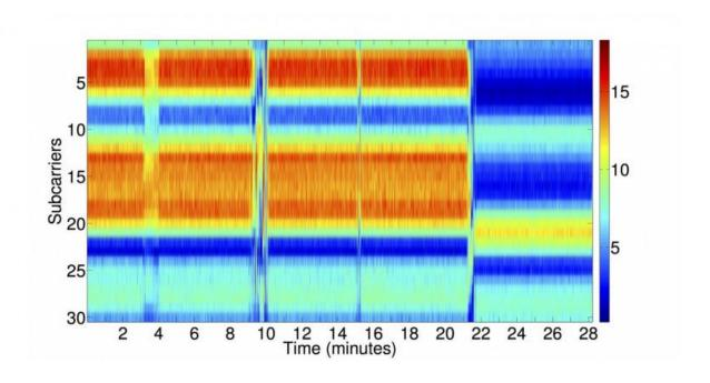
Attached image: A visual representation of the phenomenon. At 10mins and 15mins a person is moving through the environment, while at 21mins the device is being tampered with.
