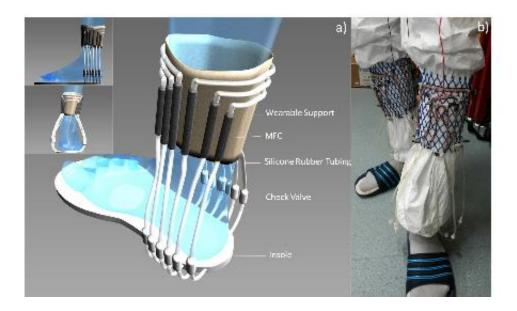
A pair of socks embedded with miniaturised microbial fuel cells (MFCs) and fuelled with urine pumped by the wearer's footsteps has powered a wireless transmitter to send a signal to a PC. This is the first self-sufficient system powered by a wearable energy generator based on microbial fuel cell technology.
