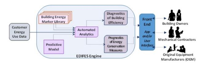
Analysis of multiple streams of data could help light commercial building owners to determine if their heating and ventilation is oversized or undersized, if the building needs new windows and insulation and more. Credit: Alexis Abramson
