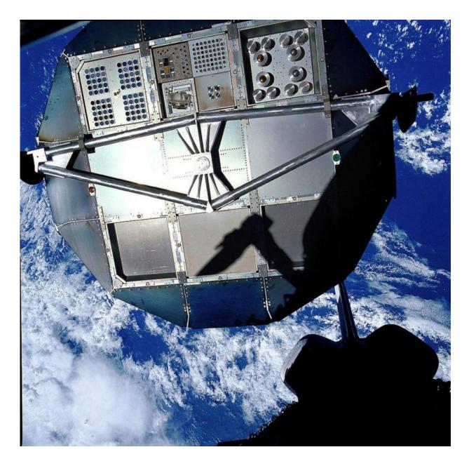
Space contamination hazard: the EXOSTACK experiment on Long Duration Exposure Facility. Credit: NASA
