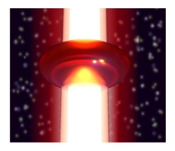
The strength and direction of light scattering can be controlled by carefully selecting a nanostructure's shape and refractive index. Credit: A\*STAR Data Storage Institute
