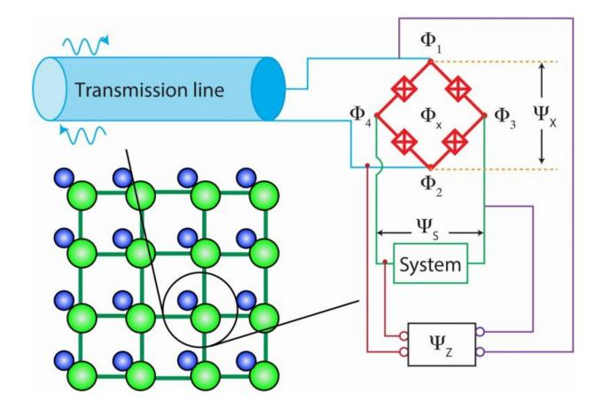
Apparatus for demonstrating chemical potential for light. The reaction of photons (represented by the green balls in the picture) with circuits (represented by blue balls) leads to a controllable thermal equilibrium of the light with the circuits. The Greek letters psi and phi refer to various modes of light.
