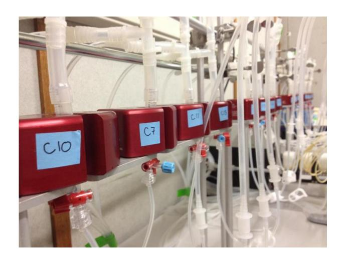
The experimental set up for the experiment published in eLife. Yeast is grown in columns, which are positioned inside strong magnets (red). Credit: Heinemann lab
