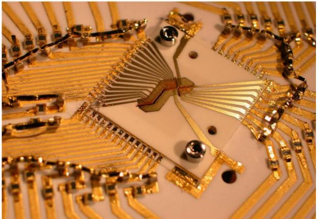
An ion trap used in NIST quantum computing experiments demonstrating logic
