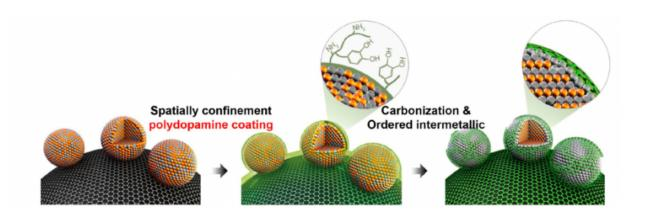
Figure A Synthesis of ordered intermetallic fct PtFe/C. Schematic synthesis diagram of carbon-supported and N-doped carbon-coated ordered fct-PtFe NPs
