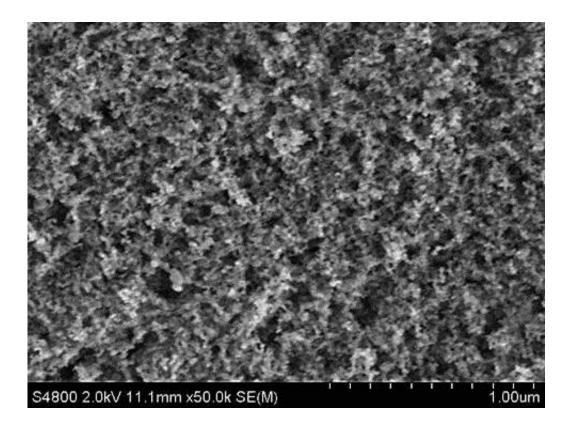
A scanning electron microscope image of a new superhydrophobic material shows the rough surface of functionalized alumina nanoparticles. Scientists at Rice University and the University of Swansea led the creation of the environmentally friendly material. Credit: University of Swansea
