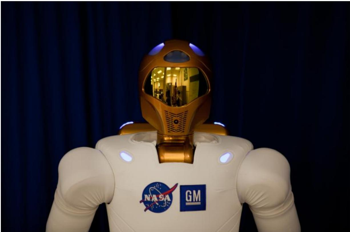
Robonaut2 – or R2 for short – from NASA and General Motors, is a robot designed to work side-by-side with people in difficult or dangerous places on Earth and in space. NASA
