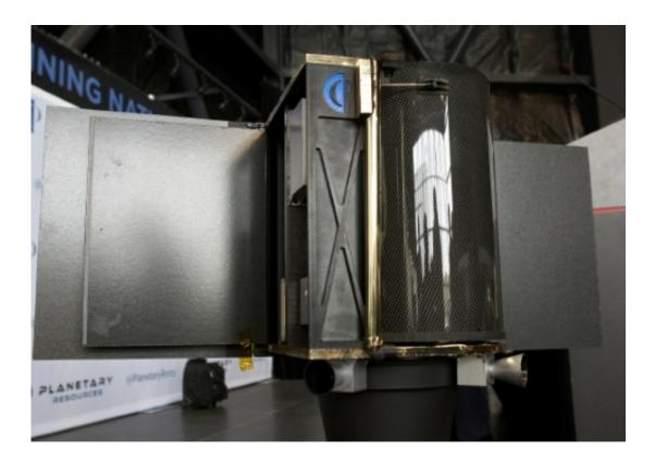
The Arkyd Seris I satellite created by Planetary Resources, which was established in 2012 to mine asteroids
