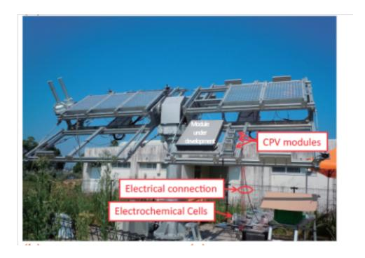
Researchers in Japan have developed an efficient way of splitting water to produce hydrogen using energy from the sun. Their technique uses a combination of concentrated photovoltaic modules with electrochemical cells, and achieves a hydrogen production efficiency of 24.4%, the highest solar-to-hydrogen efficiency yet recorded.
