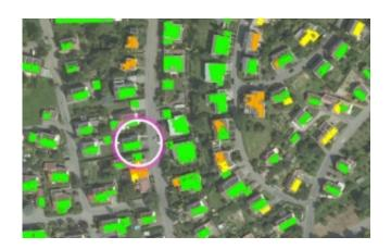
EAGLESolar project calculates the suitability of individual homes for installation of solar facilities and potential energy savings based on 3D maps, weather data, and electricity tariffs. Credit: IPF, KIT
