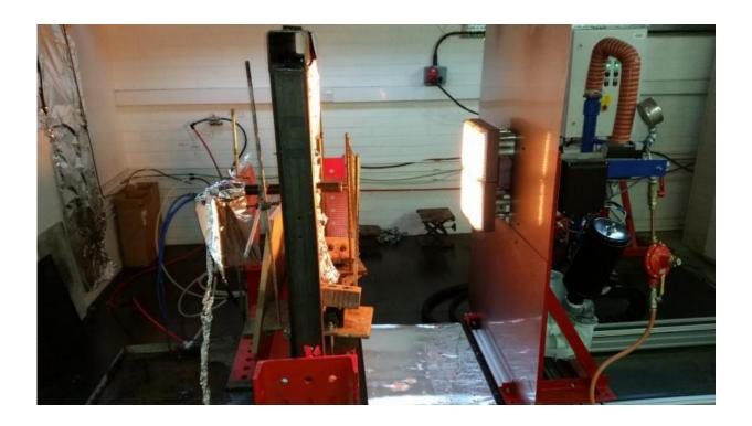
Researchers from Empa tested a SAP-containing concrete slab with a radiant heater. Some discolouring emerged at the surface of the concrete element, but no spalling occurred.
