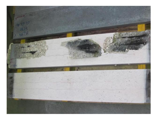
The SAP-containing concrete element resisted temperatures of about 1000 °C, and its capacitance was preserved. The slab made of concrete without SAP showed some severe spalling which reduced the loading capacity of the slab and raised the risk of a collapse.
