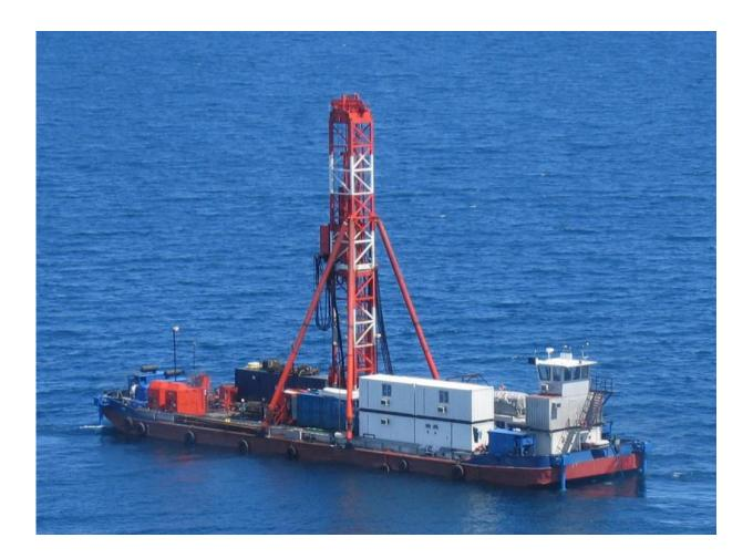
Drilling site in nearly 2000' of water on Lake Malawi. Drill cores at this location penetrated more than 1250' below the bottom of the lake. Credit: Jason Agnich, University of Minnesota Duluth.
