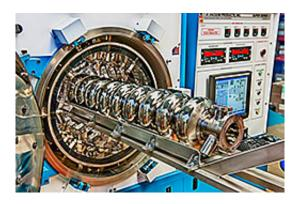
An LCLS-II-type accelerator cavity is inserted into a machine to be treated with nitrogen, a process that increases the cavity's quality factor. Credit: Fermilab
