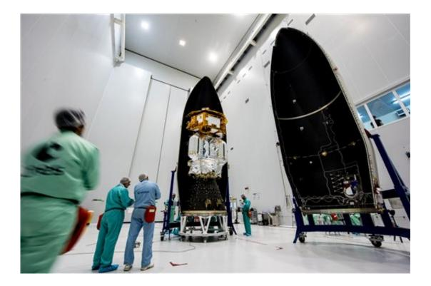
The Nov. 16, 2015 photo provided by European Space Agency ESA shows the LISA Pathfinder being encapsulated within the half-shells of the Vega rocket fairing on at the Centre Spatial Guyanais in Kourou, French Guiana. (Manuel Pedoussaut/ESA via AP)
