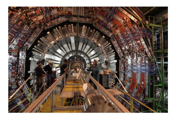
Work being carried out to upgrade CMS during the recent shutdown of CERN's Large Hadron Collider. Credit: CERN
