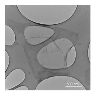
Graphene flakes in the plastics graphene compound magnified 40.000 times Credit: University of Luxembourg
