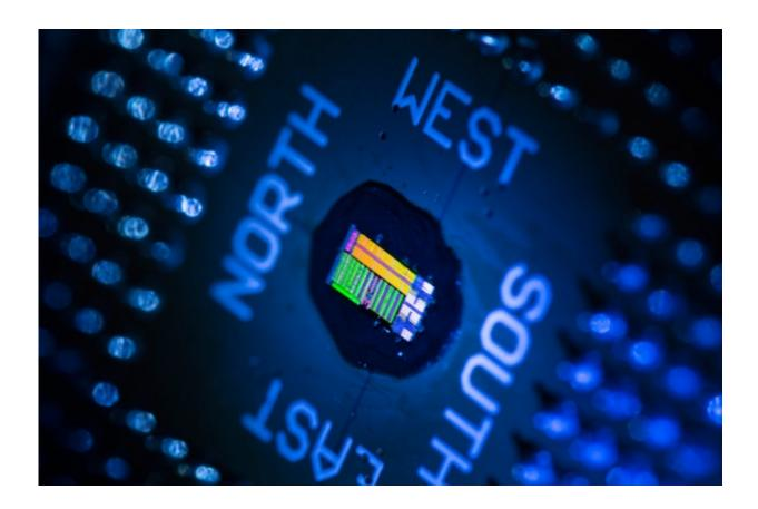
Researchers have produced a working optoelectronic chip that computes electronically but uses light to move information. The chip has 850 optical components and 70 million transistors, which, while significantly less than the billion-odd transistors of a typical microprocessor, is enough to demonstrate all the functionality that a commercial optical chip would require. Credit: Glenn J. Asakawa
