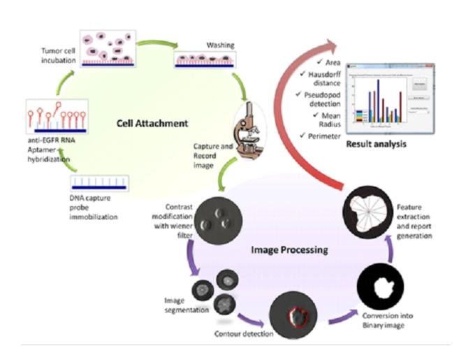
Schematic showing cell behavior tracking that starts with RNA molecules immobilized on the chip surface. The molecule binds to the overexpressed cancer receptors on the cells. Cells show distinct behavior when bound to the surface. This behavior is quantified with image processing.
