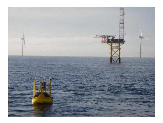
In the North Sea, wind measurement buoy with sophisticated, precise measurement technology situated in front of the FINO 1 wind met mast. Credit: Fraunhofer IWES
