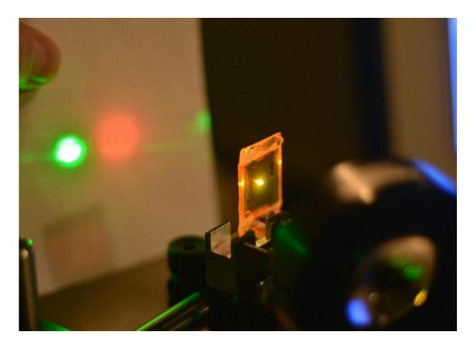
A liquid crystal elastomer is used as a mechanically tunable mirrorless "rubber" laser in the lab of Peter Palffy-Muhoray, Ph.D., associate director of the Glenn H. Brown Liquid Crystal Institute and professor of chemical physics at Kent State University. The elastomer has properties that enable it to precisely emit laser light, without the use of mirrors, while being stretched. Credit: Kent State University
